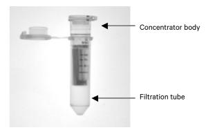
Diafiltration apparatus used for concentrating dilute antibody samples prior to starting the All-in-One conjugation protocol.
