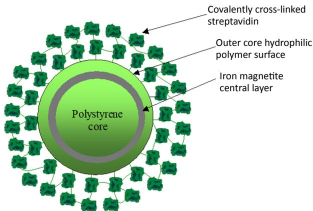
Figure 1. Cross-Section of NanoLINK Streptavidin Magnetic Beads.
